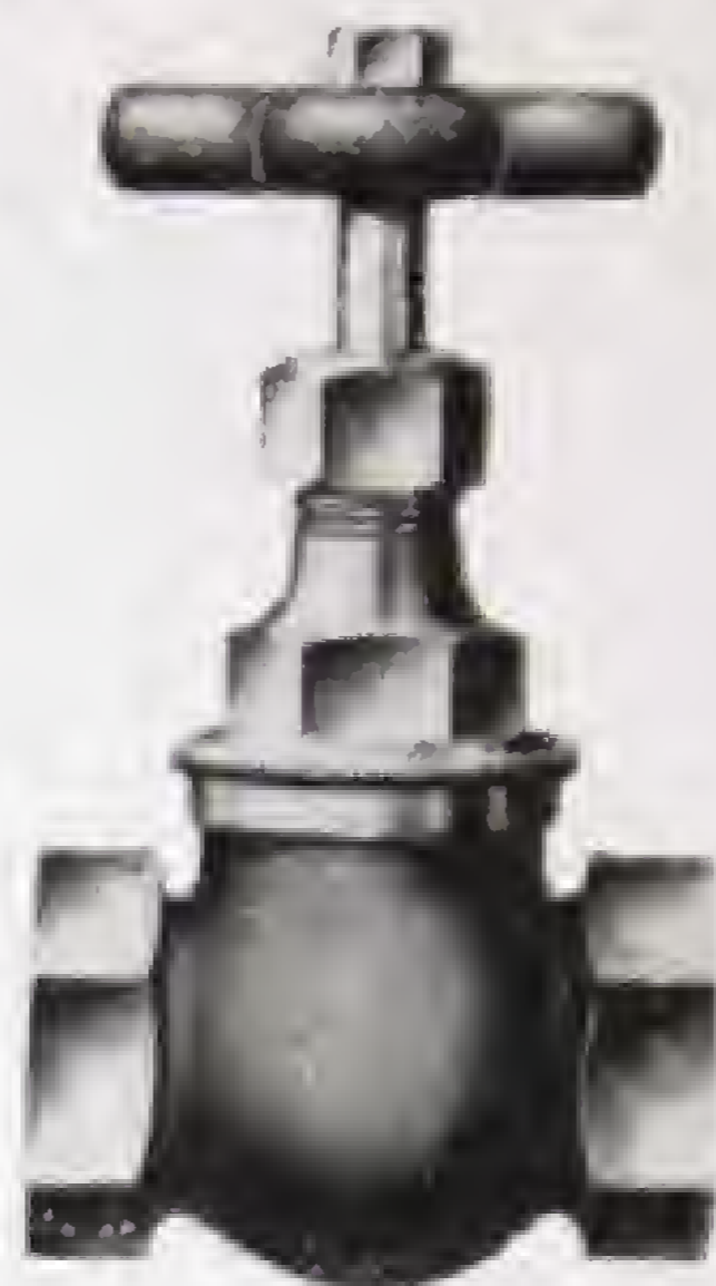
No. B 3152 WHEEL VALVE Screwed cover pattern with renewable nickel alloy clack and seat. For steam pressures up to 200 lbs. □" and a total superheat temp. of 500° F. Sizes : ¼ in. to 2 in.
